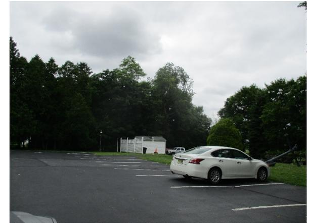
Pervious pavement can be installed in the north parking lot to help capture and infiltrate stormwater runoff from the parking lot area. A preliminary soil assessment suggests that the soils have suitable drainage characteristics for green infrastructure.
