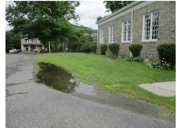
A turfgrass area to the east of the building can be converted to a bioretention system to capture, treat, and infiltrate stormwater runoff from the building's roof. A preliminary soil assessment suggests that more soil testing would be required before determining the soil's suitability for green infrastructure.
