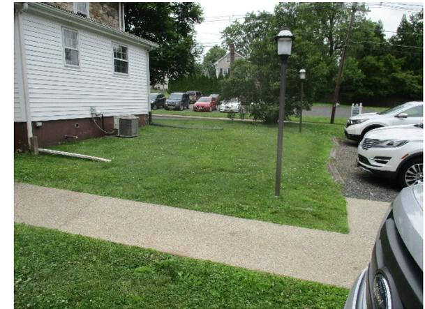
The turfgrass area north of the building can be converted to a bioretention system to capture, treat, and infiltrate stormwater runoff from the building's roof. A preliminary soil assessment suggests that more soil testing would be required before determining the soil's suitability for green infrastructure.
