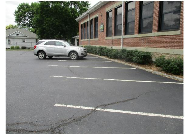
Parking spots on the west side of the building can be converted to pervious pavement to capture and infiltrate stormwater runoff from the building's roof and the parking lot. Mirrored bioretention systems can be installed to the east of the building to help capture, filter, and infiltrate stormwater runoff. A preliminary soil assessment suggests that more soil testing would be required before determining the soil's suitability for green infrastructure.
